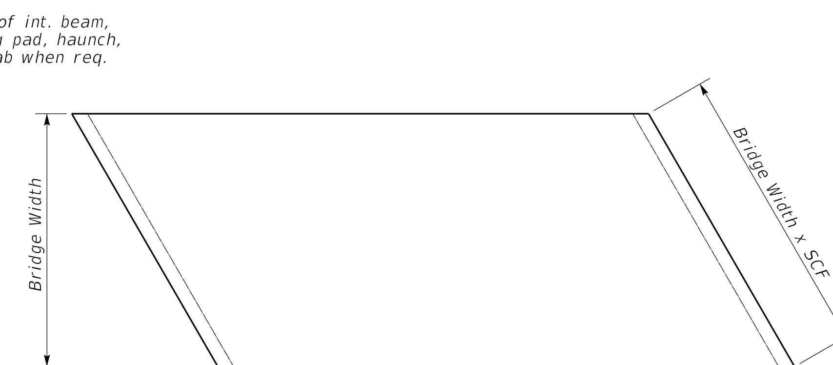
PLAN OF SUPERSTRUCTURE SLAB
